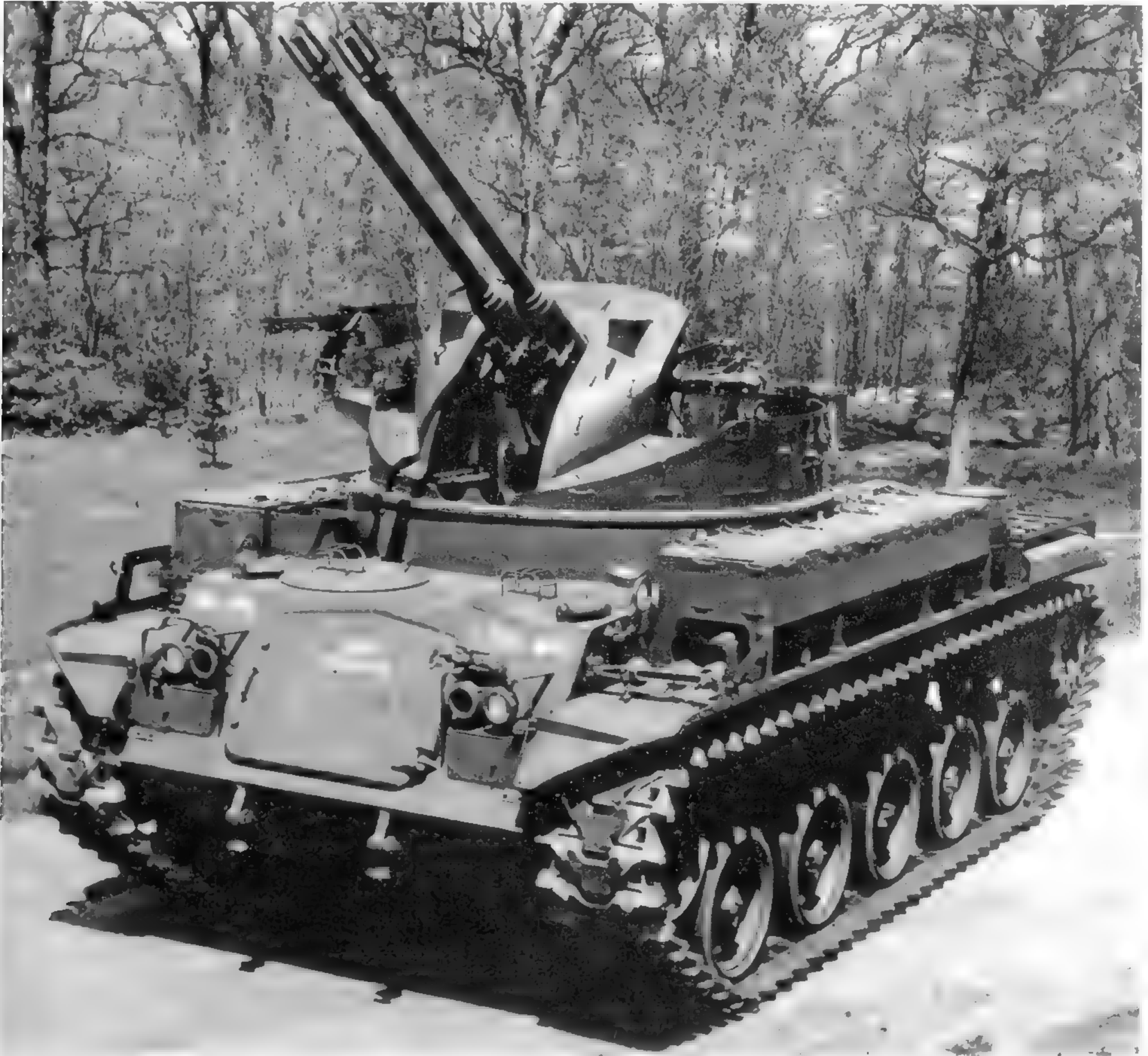
The Bofors cannons on M42 vehicles had a maximum rate of fire of 120 rounds per barrel per minute. The stowage boxes on top of the fenders provided space for some of this ammunition. (U.S. Army photo)
